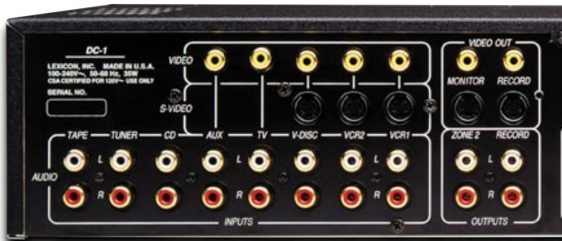
The rear panel of the DC-1 reveals a wealth of facilities, including full audio/video switching for five inputs (including three S-video) plus three additional audio inputs, and multiple coax and optical digital (S/PDIF) connectors. On the output side, there are both monitor and record video and S outs, the monitor output including system menu video overlays if desired;
