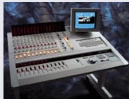
*The Lexicon Opus was one of the first Digital Audio Workstations available, with the ability to record, mix and assemble several simultaneous digital audio tracks into a composite mix of the highest quality – without the use of tape.*
