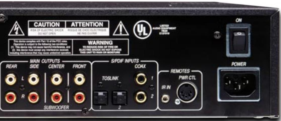
independent outputs for recording and for a second room; and a full complement of main front, side and rear line level outputs plus center and subwoofer feeds. A DIN connector provides 12v triggers to control of external devices such as TVs, projection screens or lighting controllers, and a facility is provided for direct infra-red remote control input.
