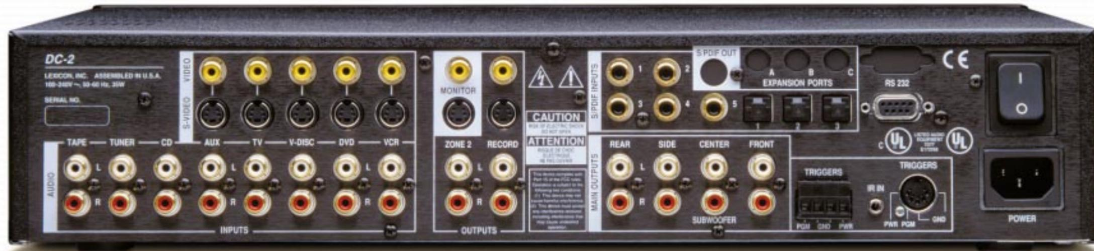
The rear panel of the DC-2 reveals a wealth of interface capabilities, including full audio/video switching for five A/V sources plus three additional audio inputs, and multiple coax and optical digital (S/PDIF) connectors. On the output side, there are both monitor and record video and S outs, the monitor output including system menu video overlays if desired; independent outputs for recording and for a second room;
