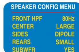
Parameters of the DC-2 can be set up with ease, thanks to a simple on-screen menu system. Menus are optionally superimposed on video from the Monitor output, and are controlled with dedicated buttons on the remote.
