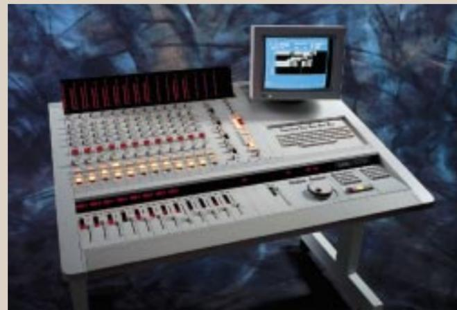
The Lexicon Opus was one of the first Digital Audio Workstations available, with the ability to record, mix and assemble several simultaneous digital audio tracks into a composite mix of the highest quality – without the use of tape.
